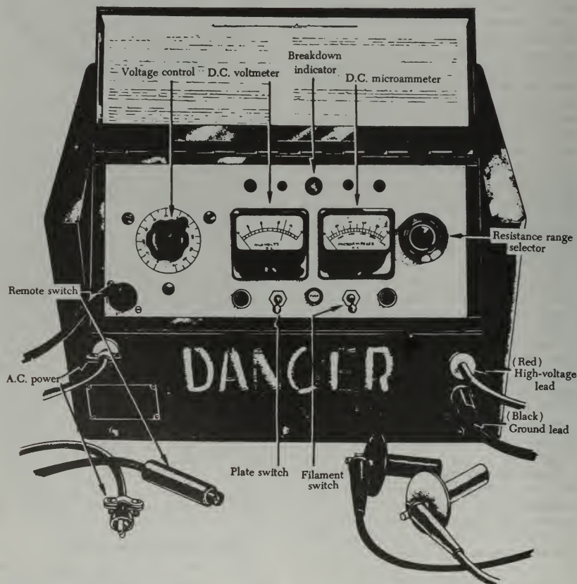
FIGURE 4-70. High-tension ignition harness tester.
